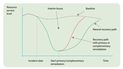
Figure 3: Illustrating baseline, initial damage, interim loss and remediation measures
